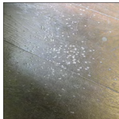
High traffic stiletto heel indentation of a moderately hard timber
